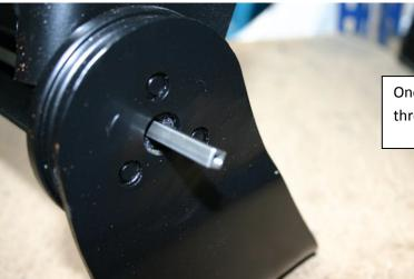
Once aligned the bar can be pushed through the frame.
