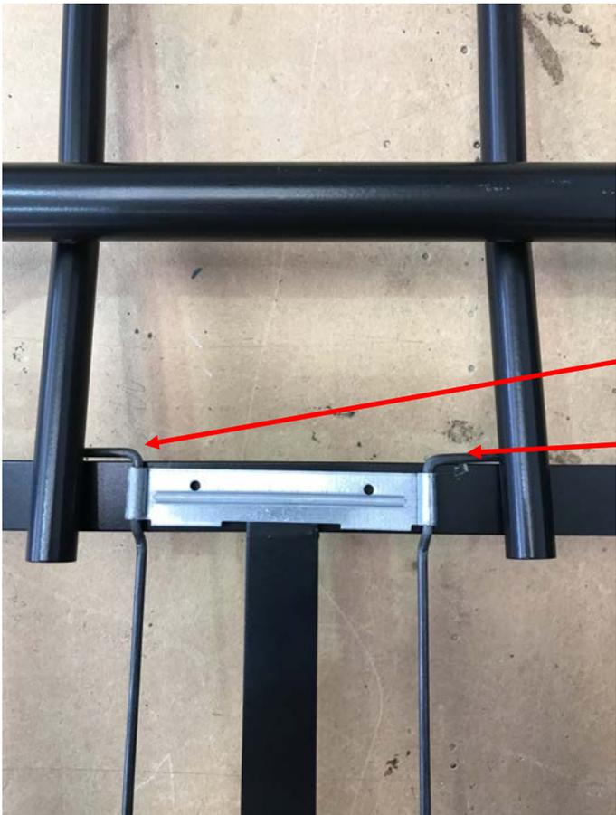
If you are fitting the wire frame to a frame that features an integral headrest, ensure the top section of the wire frame is pushed through to the front of the headrest frame before attaching cable ties
