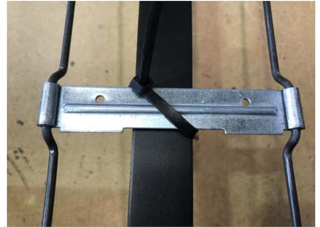
Central section of wire frame fitted to rear of squab frame
