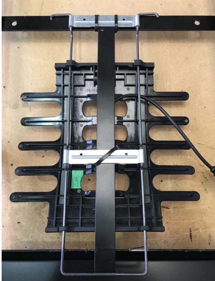
The fitted lumbar assembly should look like the picture on the left. This is shown with the adjuster wire ready to fit into the right-hand side of the squab frame.
