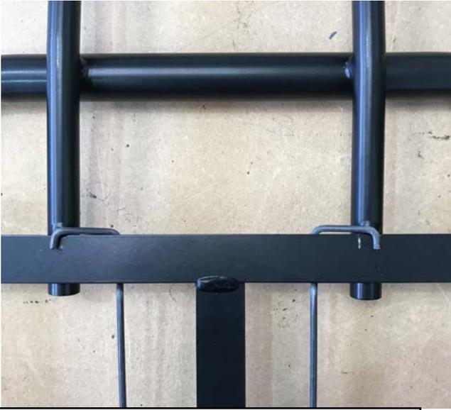
Front of squab frame on integral headrest type showing wire fitting.
