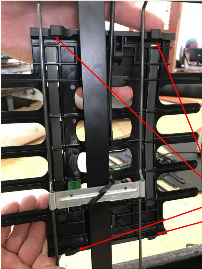
Next take the lumbar assembly and slide on to the wire frame from the **FRONT** of the seat frame. Ensure the adjuster actuator wire is pointing **UP** and is loose enough to allow it to be fitted on either the left or right-hand side of the squab frame as required.
