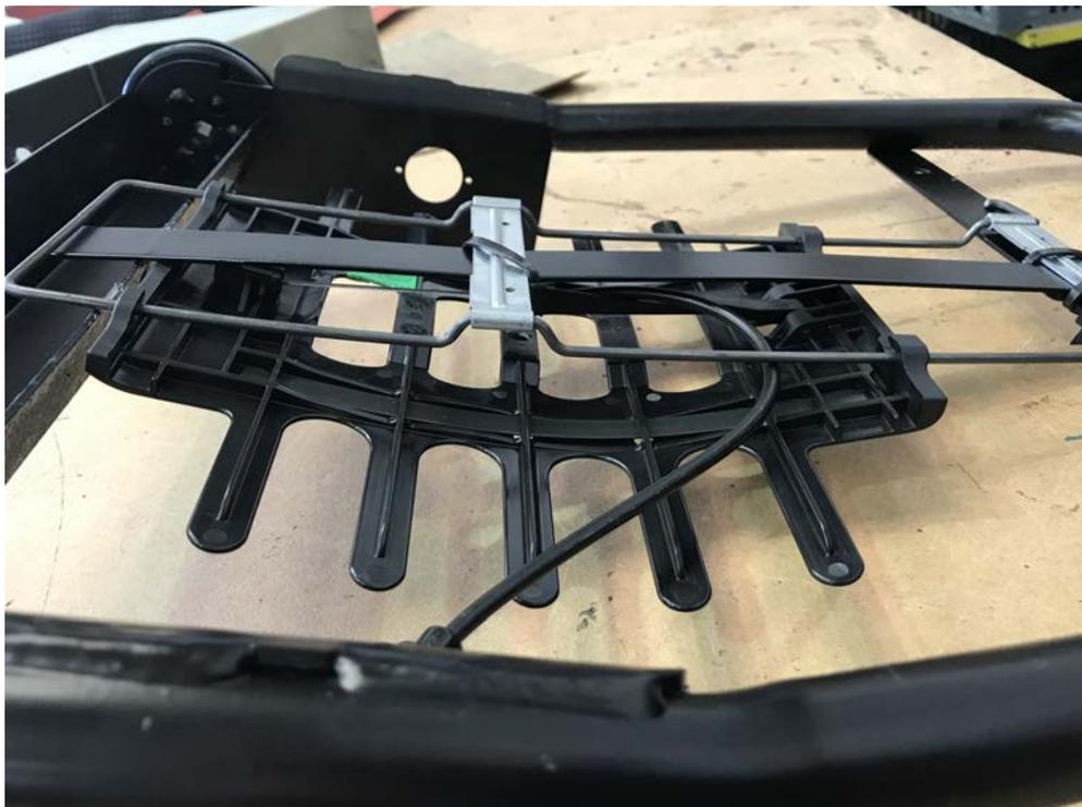
Rear view of squab frame with lumbar assembly completely fitted including actuator wire.
