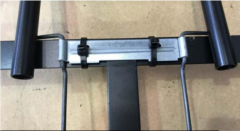
Rear of squab frame on integral headrest type showing wire and cable ties fitted.
