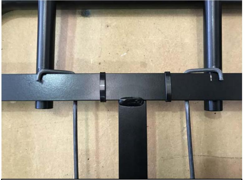
Front of squab frame on integral headrest type showing wire fitting with cable ties fitted.
